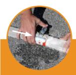
Place the hose-bandage left or right from the leaking spot on the hose and place the trigger in one of the two size settings, depending on the hose.
